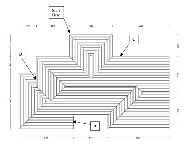
To draw up the roof we need to split it up into two sections. The above section is the majority of the roof and we will draw it up first.
