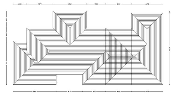
From here we use the command **Mod-Roof** | **Advanced** | **Intersect-Planes**. The software will then intersect all the roof planes giving you the following result.
