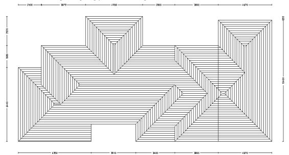
One more thing left to do and that is to delete the unwanted gable end in the middle of our roof. First of all we need to delete the plane tag associated with it. The easiest way to do this is to go to **CAD** | **Surface** | **Plane** | **Delete** and drag a box around the gable end, right click the mouse and confirm the delete. When you have done that go to the normal **delete** from the main menu and delete the unwanted lines. There will be three of them. That completes our job.
