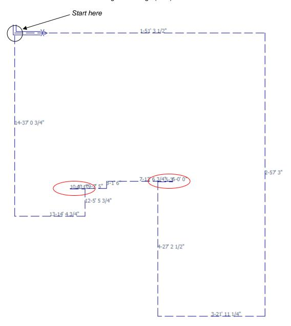
3. Remember to close square so that you can check the wall measurements against the plan) and then set the pitch and overhang. It is easier to do these roof shapes (with barge lines) with zero eave overhang. If you have a plan with wall measurements, then add the overhang to the line lengths.
