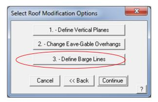
5. You usually have at least two barge lines, one going up and one going down. Select each barge line in turn and observe that the eave height at the corner is displayed. Do not select them the lines more than once.
