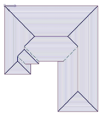
Draw your wall outline taking account of the need for barge lines. Subtract the length of eave that is tucked under the front roof, and add this later using Mod-Roof > Extend Barge.
