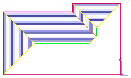
5. Next draw a new gable end up using the Smartlines option Insert-Freehand. I snap to the end of the new line (using middle mouse button) and then type in iy(length), (incremental length, in the Y axis) which is the end of the line and select Gable as a
