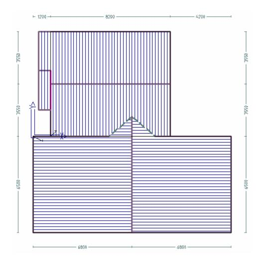
We need to draw a flat roof in front of our split gable. Select Construct Roof - Track Outline - Plane Roof.
