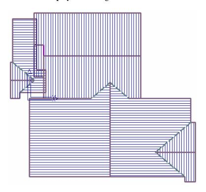
We then need to draw the remaining parts of our first story by tracking plane roofs. Select **Construct Roof > Digitise Outline – Plane Roof**. Constrain angles to 90 as we are drawing square roofs with no non 90 degree corners.
