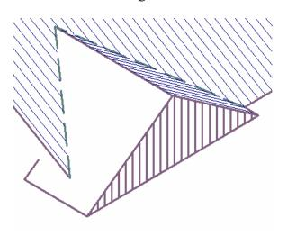
Select **Draw Freehand** and snap to top of our moved gable line then the bottom of the dormer valley. Select **Apron** for line type
