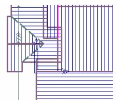
Select **Modify roof > Advanced > Merge Planes** and merge this plane with the one under it like you did with the plane on the other side of the roof.
