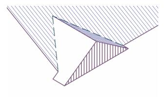
Select **Move** and select the small gable end we wish to move. Type on keyboard ix-900 and press **Enter**. This moves our gable end back 900mm.
