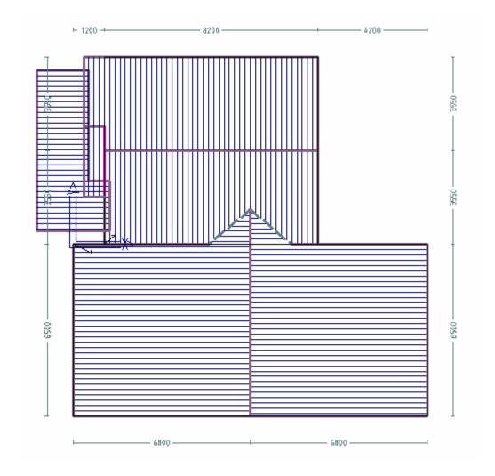
As the dormers on this model wrap around the eave, we will draw them as gable roofs and intersect them into the main roof. Select **Construct Roof > Track AutoRoof - Hip Roof**
