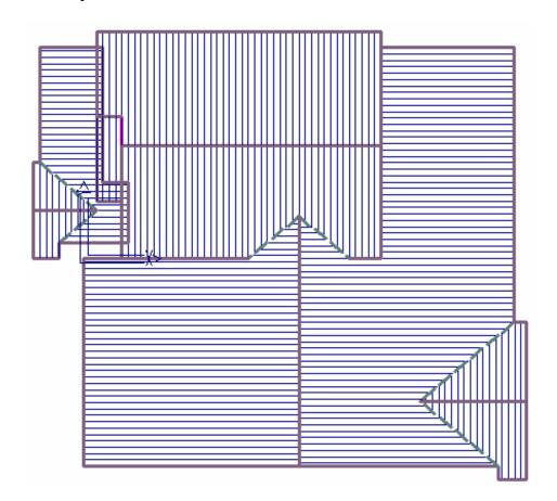
A small section of roof needs to be added to the left side of our first story. **Construct Roof > Digitise Outline – Plane Roof.** Snap to the top left corner of our first story under our veranda etc then snap to the right corner beside it that joins the wall of our second story. Type on keyboard iy700 and press enter. Right click and close square. 3000 eave height and 30 degree pitch and select your pitching line on left side.
