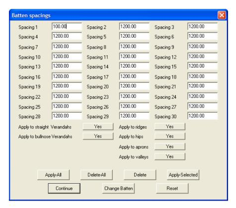
Select **Apply all** to apply the battens then **Continue** and then select **Generate** to get a purlin cutting list.
