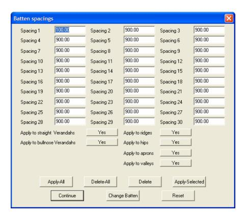
If you need to reset batten spacing's, select the **Reset** button and reset spacing to what you require, in this example, reset to 1200 then change the first spacing to 100.00
