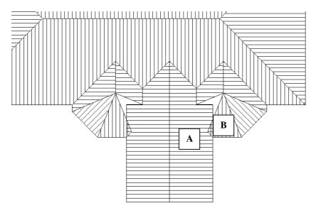
Just to make it a little easier we will turn **Off** the wall lines under **Utilities** | **Set-Display**. From here we need to delete planes **A** and **B**. We should then go into an **Iso** view as it is easier to see what is going on.
