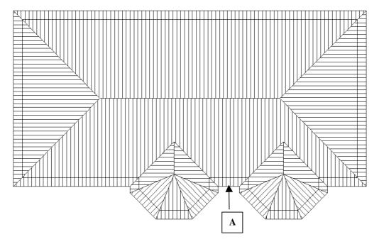
First, draw up the roof part in question without the projected carport, as shown above. Then add in the carport using the dormer command and selecting eave line **A**. Your roof should look similar to the one below.
