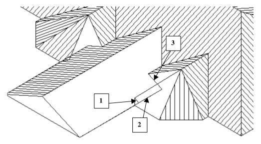
Now delete lines 1, 2 and 3. (When you select line 2 it will start flashing, select the shorter of the two lines.)
