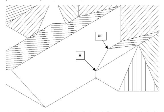
The final modification we need to do is to insert a line from point **ii** to point **iii**. Go to **Mod-Roof** | **Advanced** | **Ins-Line** | **Free**, and "**Snap**" to points **ii** and **iii**. Your roof should look like the following.
