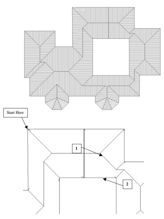
To draw up the roof start where shown and go right until you get to about the middle of the courtyard. From here go down **line 1**, until you get to the eave of the courtyard. Then go left to the inside left wall of the courtyard, for example left **3000mm**, then go down **7000mm**, then right **7000mm**, then up **7000mm**. Now we need to go left far enough to leave a gap of **50mm**, in my example **3950mm**. Finally we need to back up the distance that we came down.
